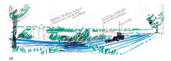
The road becomes a drain and the heavier the rainfall is, the more the road is invaded by water and the more the flow of water and silt accelerates. The overflowing river turns into a destructive torrent.
